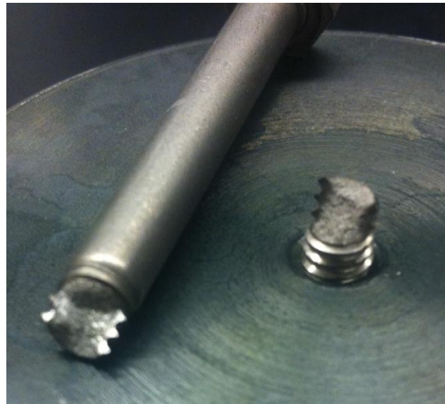
Figure 14: A286 Fastener Failure
