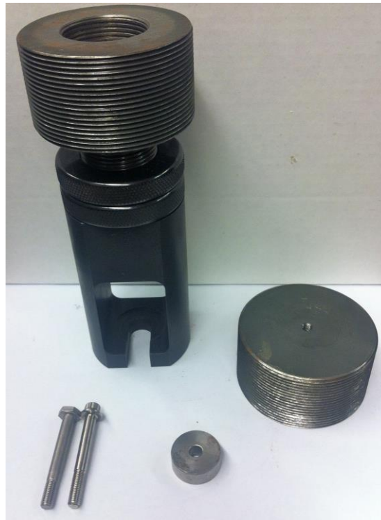
Figure 7: Custom Test Fixtures, Gripper, Washer, and Fasteners
