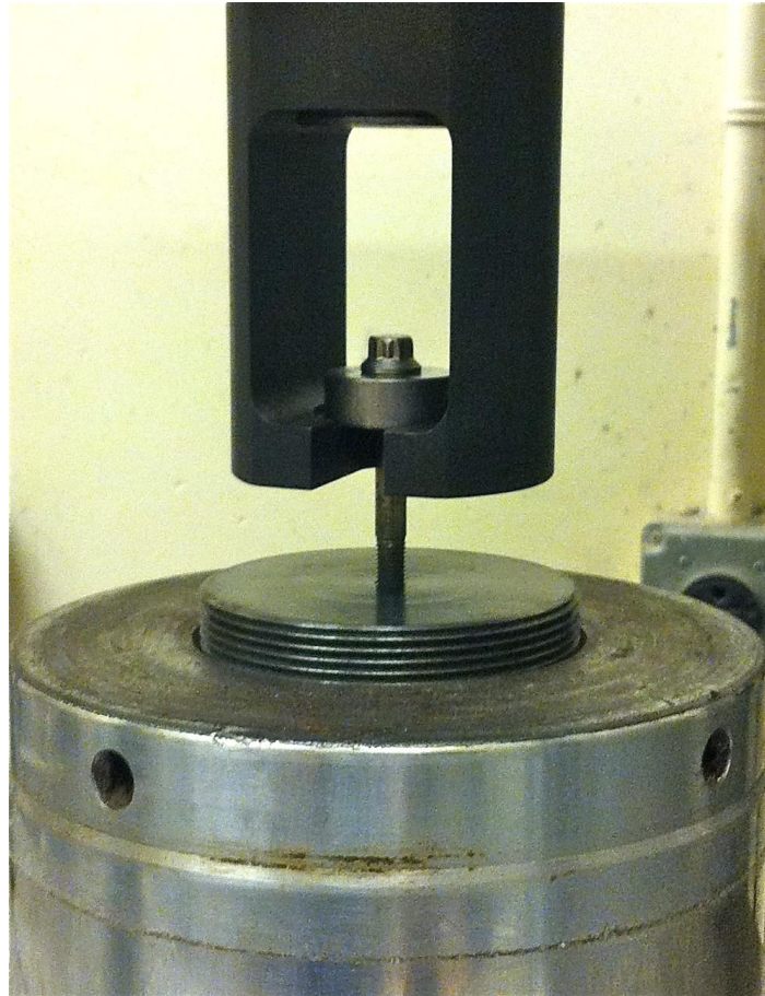
Figure 6: MTS Gripper with Tensile Specimen Ready for Testing
