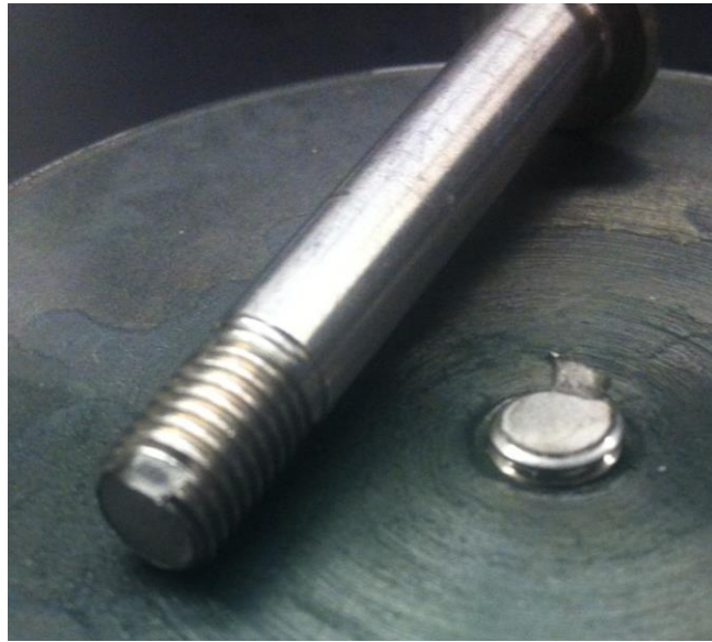
Figure 13: Titanium 6-4 Fastener Failure
